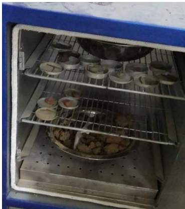
Figure 3: Oven drying of soil sample
