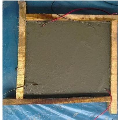
Figure 2: Specimen after casting
