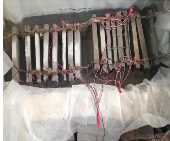
Figure 5: Specimens in Corrosion Cell
