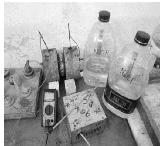
Figure 4: Rapid chloride permeability test setup
