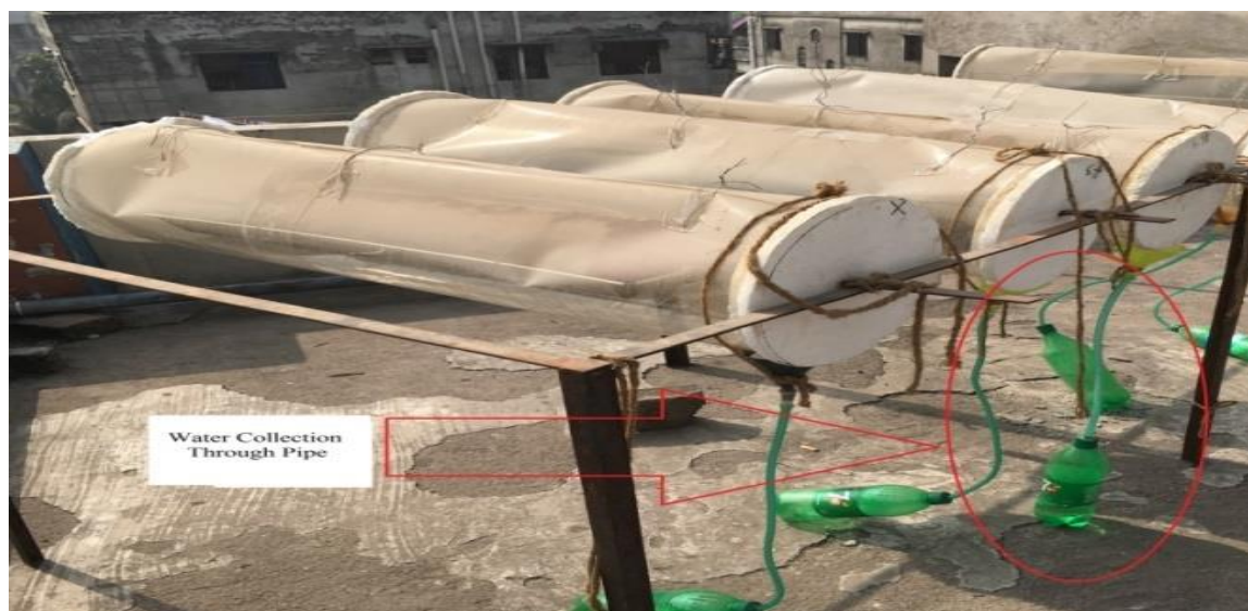
Figure 6: Collection of Distilled Water from System
