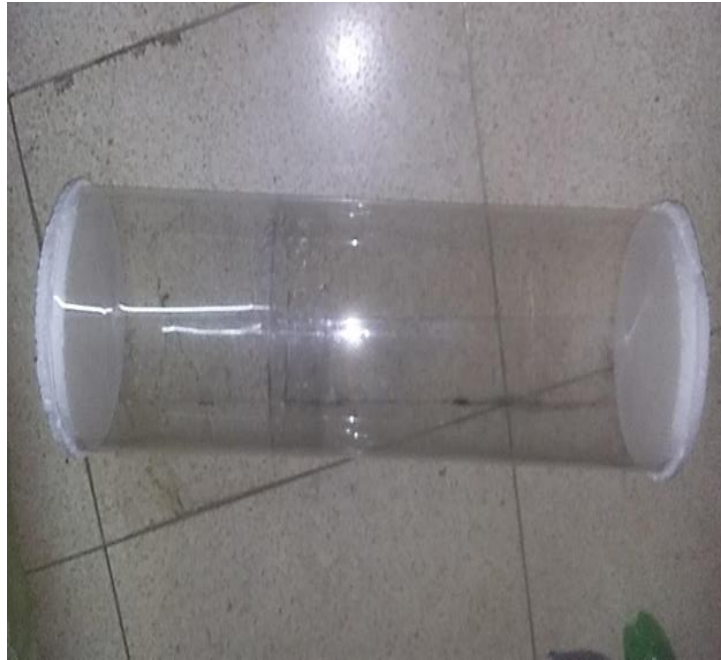
Figure 2: Rolled TPS Sealed With CorkSheet Disc at Both End.
