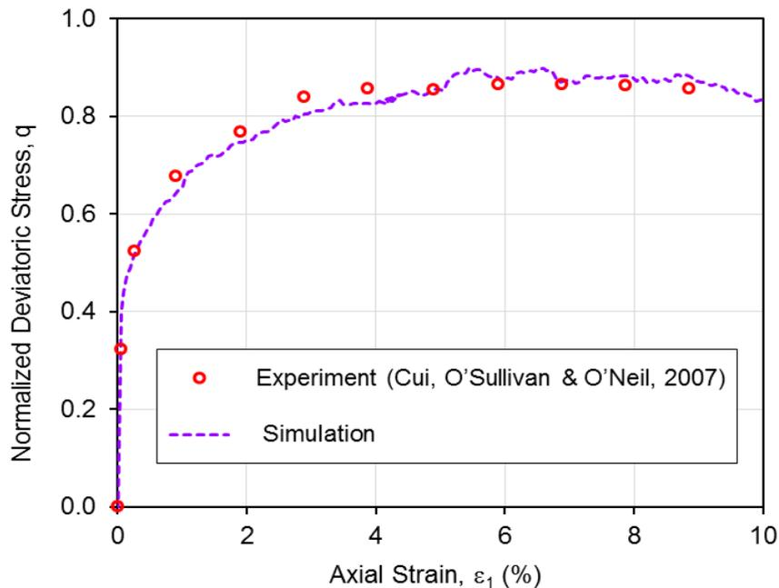
Figure 2: Comparison of the simulated stress-strain behavior using DEM with the experiment reported in Cui, O'Sullivan & O'Neil (2007)
