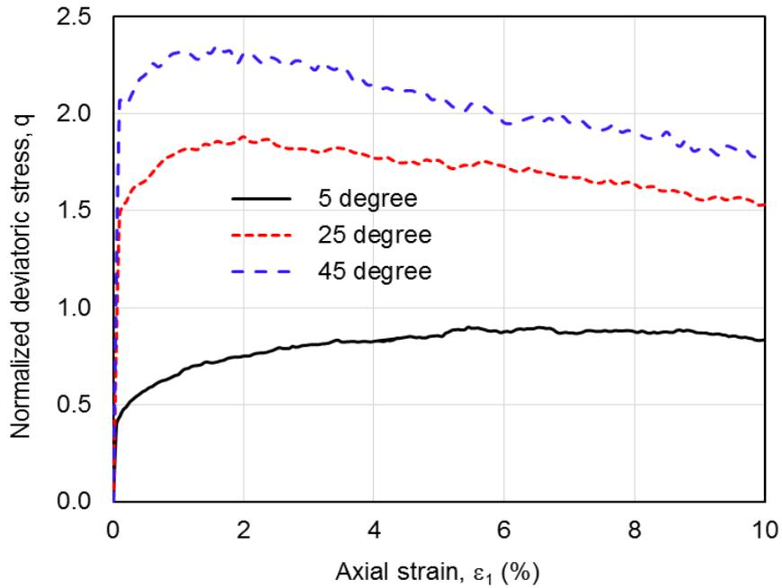
Figure 3: Stress-strain relationship for varying interparticle friction angle
