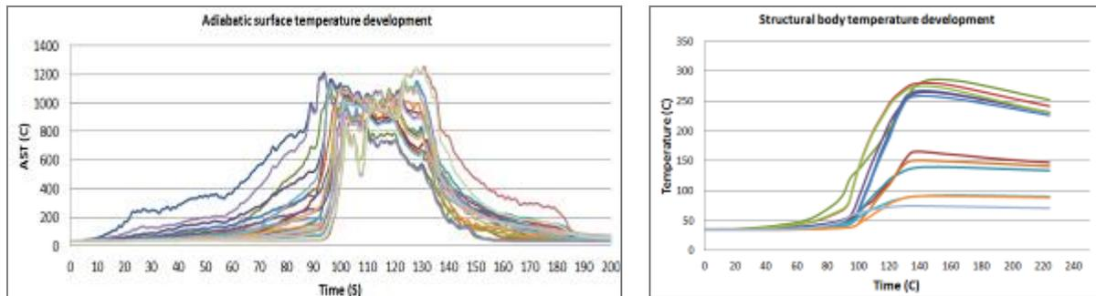
(a) Adiabatic surface temperature development of the structure (b) Body temperature development of the system
