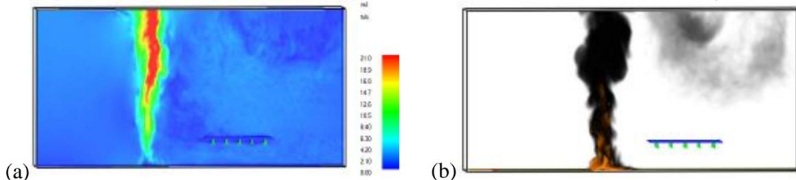
Figure 17. Velocity field and flame and soot distribution; (a) Wind velocity on the middle plane of the domain, (b) Fire plume and soot generation
