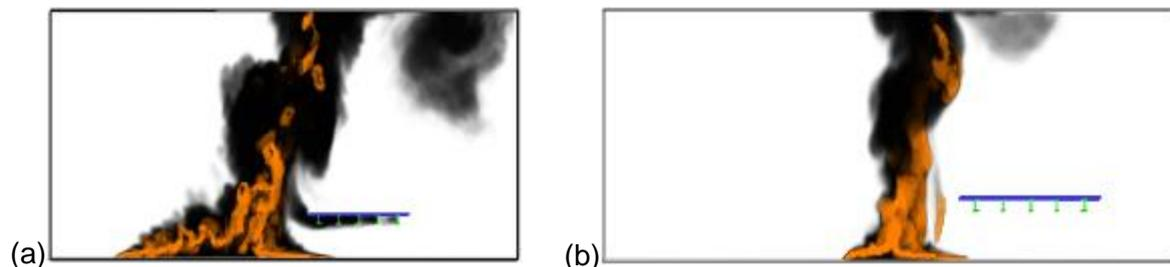
Figure 19. Fire plume and soot generation; (a) Case B, (b) Case C
