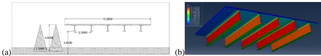
Figure 16. Models set up; (a) Distribution of surface and elevated vegetation fuel around the structure, (b) Temperature development of the heat transfer model in Abaqus FEM.
