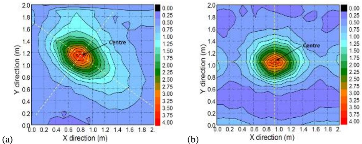
Figure 10: Distribution of flux density of spray for multi-orifice nozzle for case A; (a) Experimental, (b) Numerical.
