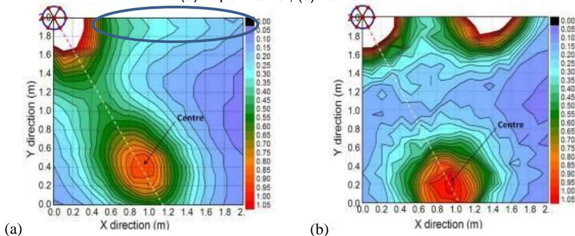
Figure 11: Distribution of flux density generated by a multi-orifice nozzle for case B; (a) Experimental, (b) Numerical.
