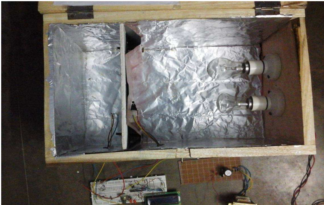
Figure 7: Setup of the specimen in the heat resisting experimental box
