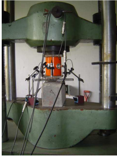
Figure 5: Loading arrangement (LA)
