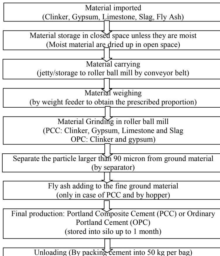
Figure 1: Total Process Flow Diagram of Cement Manufacturing in SSCML
