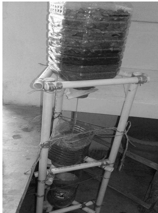
Figure 2: Practical view of the developed domestic grey water treatment unit.
