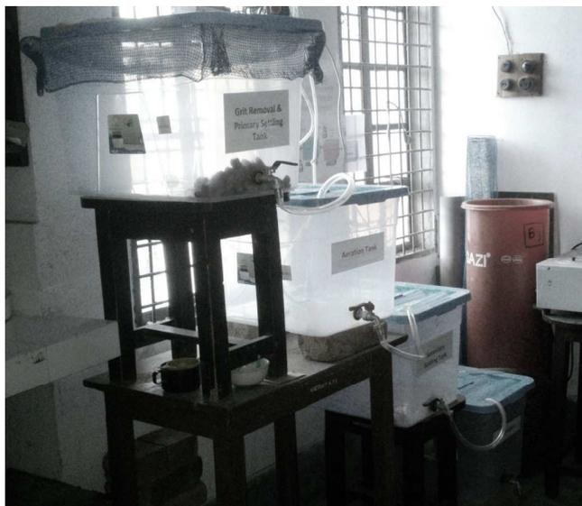
Figure 3: Photograph of experimental set up for the pilot-scale treatment plant
