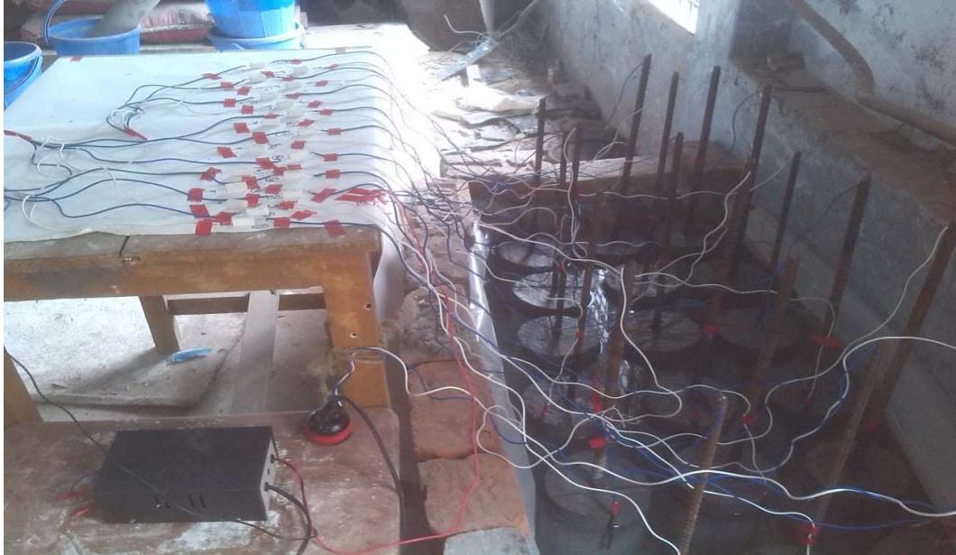
Fig. 3: Test setup for corrosion acceleration
