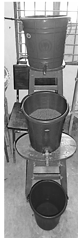
Figure 3: Experimental set-up of developed filter unit.
