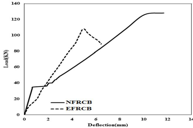
Figure 8: Comparison load-deflection behaviour of Retrofitted RC beam
