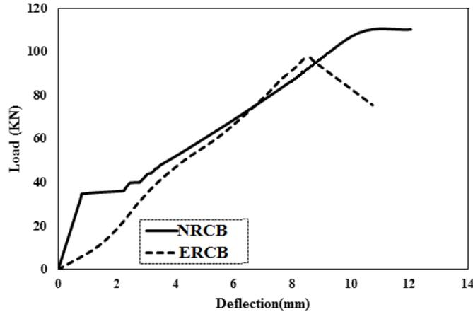
Figure 7: Comparison load-deflection behaviour of RC beam
