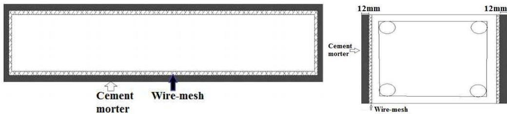
Figure 2: Top view and Cross Section of Retrofitted RC beam (one layer of wire mesh)
