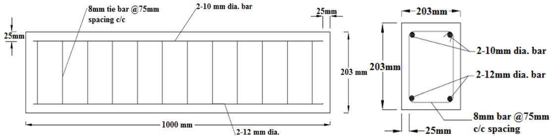
Figure 1: longitudinal section and cross section of beam
