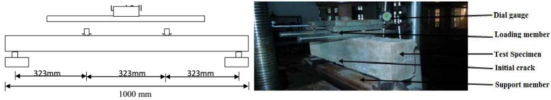
Figure 3: Experimental setup for testing of beams
