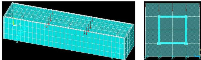
Figure 6: Isometric view and Side view of constrained model
