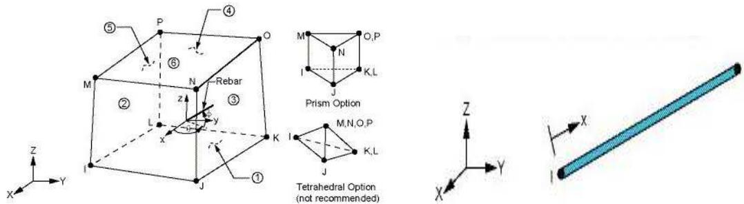
Figure 4: SOLID65 geometry and LINK8 geometry
