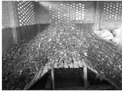
Figure 4: Trapezoidal composting pile
