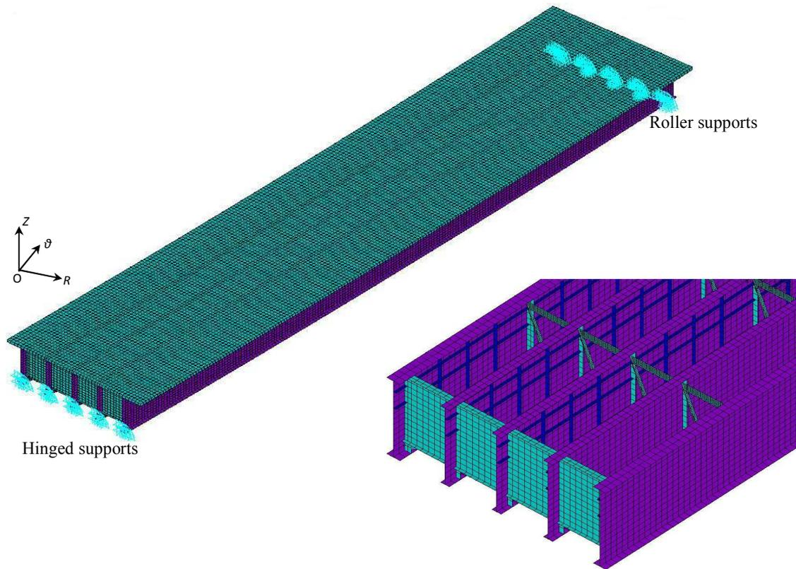
Figure 2: Finite element model of Kita-go Bridge
