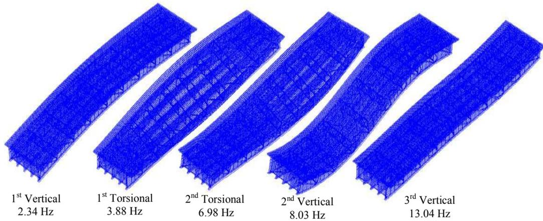
Figure 3: Natural frequencies and mode shapes of one span Kita-go bridge
