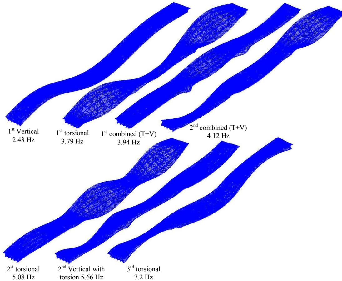
Figure 5: Natural frequencies and mode shapes of three-spans Kita-go bridge
