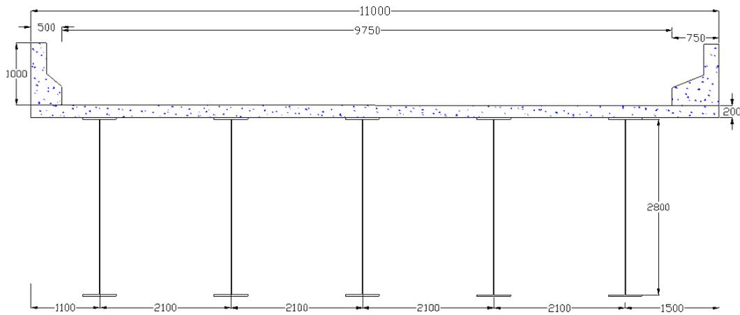
Figure 1: Cross-section of studied bridge (mm)
