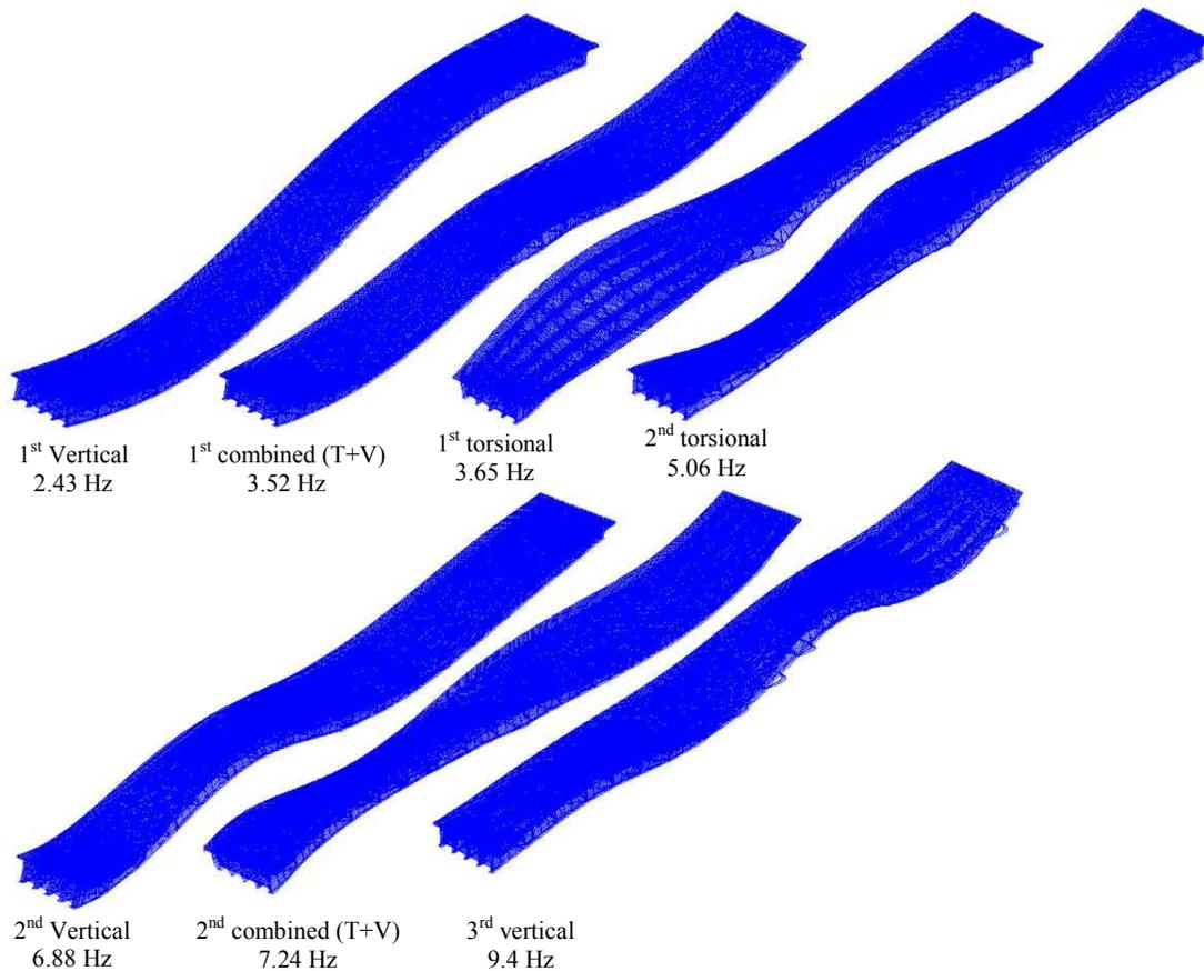
Figure 4: Natural frequencies and mode shapes of two-spans Kita-go bridge
