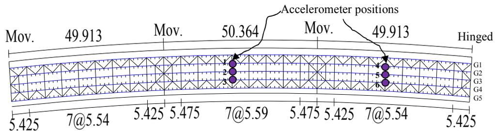
Figure 6: Accelerometer positions of three-spans Kita-go bridge
